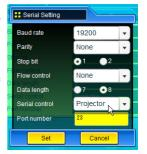
Setting for controlling the projector from the computer through the LAN port.
